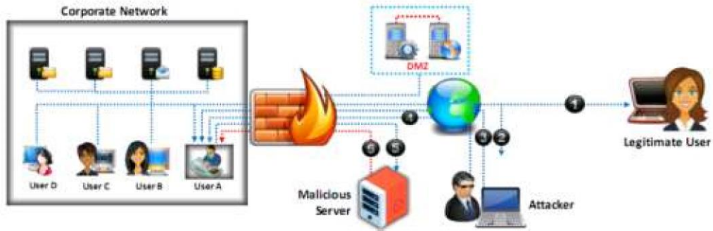
Bypassing firewall through MITM attack
